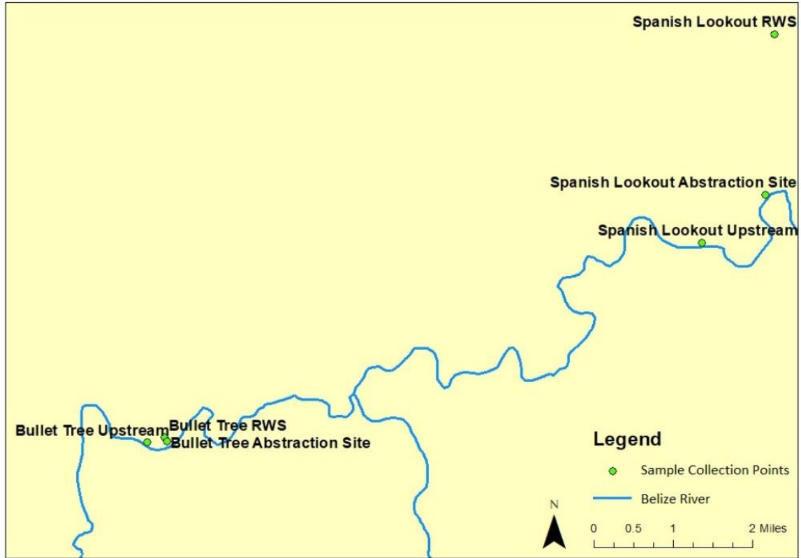
Figure 3-2 Zoomed in map of sample collection sites, showing the three different sampling points in each village. RWS stands for rudimentary water system. Abstraction sites are locations at which drinking water systems pump water from the river.
